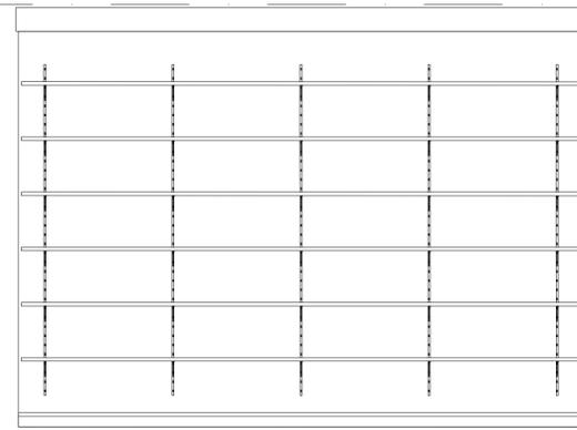
STORE ROOM WALLS 15mm PLASTERED AND PAINTED FULL HEIGHT TO ACCOMMODATE STEEL BRACKETS, TO ARCHITECTS APPROVAL
