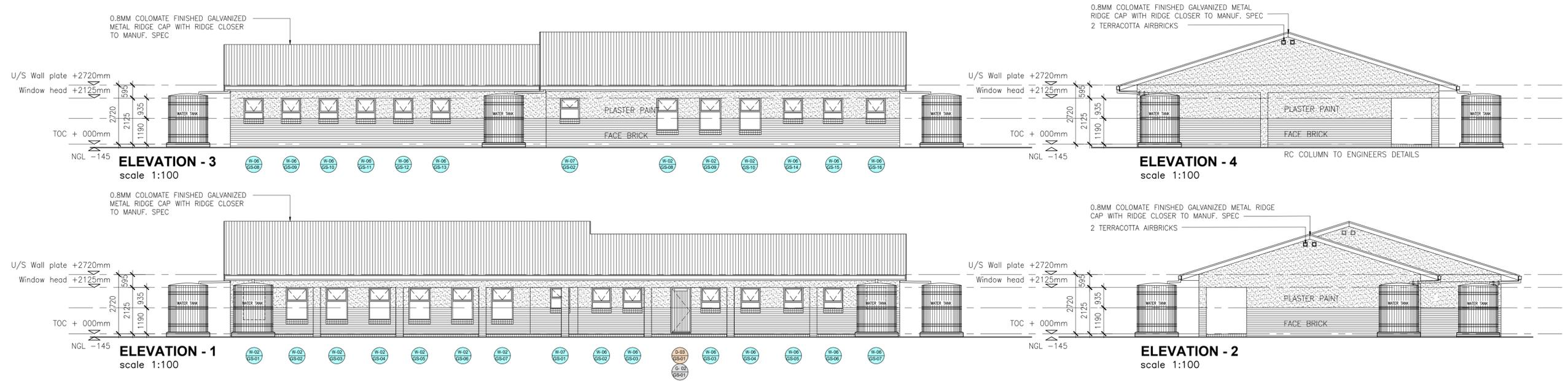
0.8MM COLOMATE FINISHED GALVANIZED METAL IFR PROFILE ROOF SHEETING @ 17,5' ON INSULATION ON 76x50mm S.A PINE PURLINS @ 1050mm C/Cs ON PREFABRICATED TIMBER TRUSSES TO ENG'S DETAIL AND SPEC.
