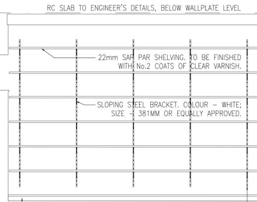
RC SLAB TO ENGINEER'S DETAILS, BELOW WALLPLATE LEVEL
