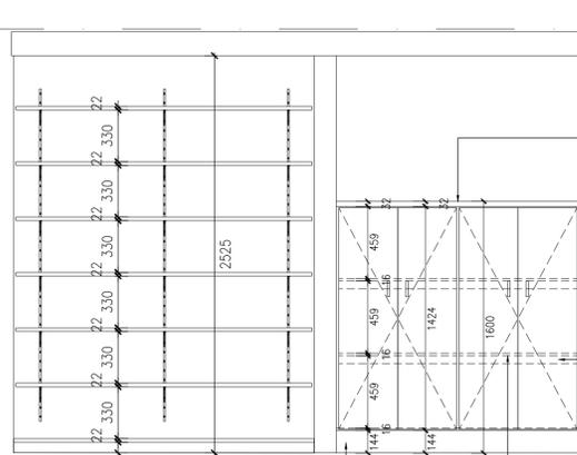
32mm THICK POST FORMED FORMICA WORKTOP WITH TOP HALF ROUND EDGE TO ALL EXPOSED EDGES. COLOUR: TO ARCHITECTS APPROVAL.
